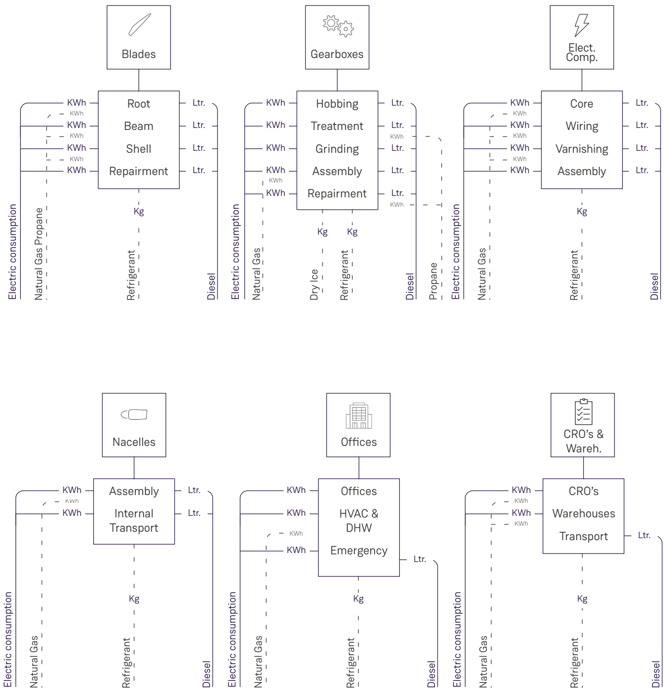
Figure 4: Overview of the emissions associated with the processes undertaken by Siemens Gamesa.
