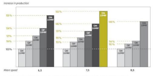
\* NOTE: theoretical production calculated for k=2, density 1,225 kg/m3, with average speed at hub height.
