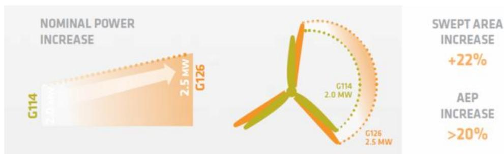
The development of the G126-2.5 MW fits into the evolutionary and modular approach that characterises the company's R&D efforts. The turbine has a 62-metre blade, a new variation on the 56-metre blade, which has been installed and widely validated on Gamesa projects using the G114 turbine; it maximises output while producing low levels of noise. It also shares the electricals with the 2.5 MW models in the platform.
