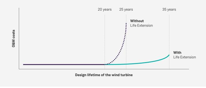
The lifetime 0&M costs of the wind turbine are reduced dramatically by applying Life Extension.
