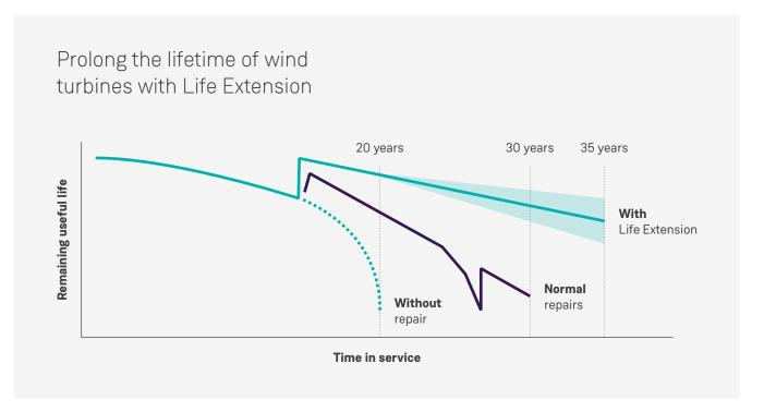
After 20 years without repairs, the useful life of the fatigue components is reached. With normal repairs after the first failure, the remaining useful time will be prolonged, but will never reach the optimized lifetime of a wind turbine where you have implemented the Life Extension service. By having regular inspections, you prevent failure and therefore increase revenue.
