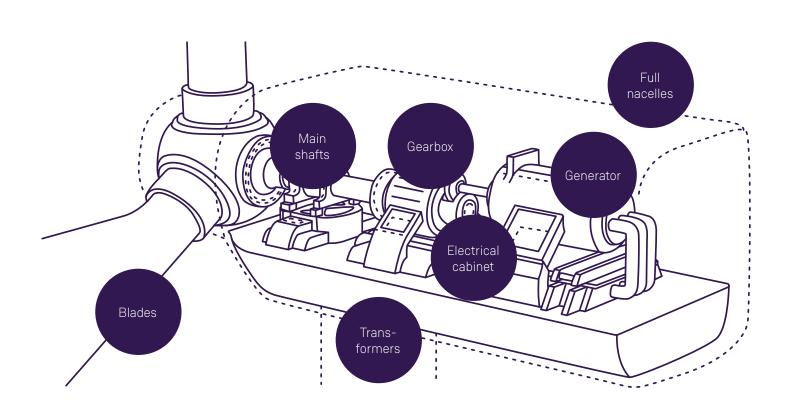
Siemens Gamesa offers repair services for the majority of major components in the wind turbines. From gearbox, generator, main shaft and transformers to blades and full nacelles.
